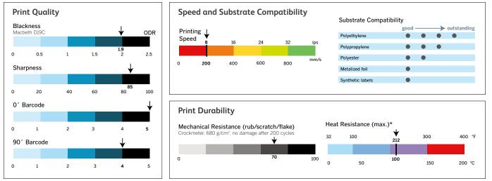
\*Extreme temperature ribbon has characteristics promoting enhanced adhesion to allow the print to withstand high temperature exposure. Videojet evaluation of observed performances of the Standard Ribbon with optimized printer setting and receptors.
